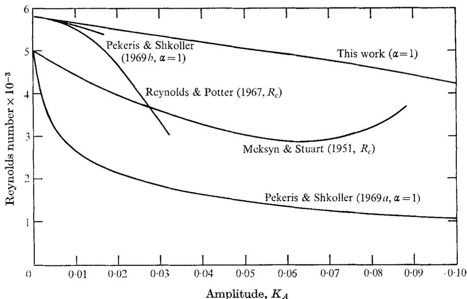
FIGURE 7. Comparison of critical curve with earlier work.
