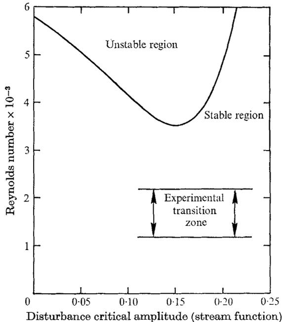
FIGURE 6. Critical behaviour for finite amplitude disturbances ( $\alpha = 1$ ).
