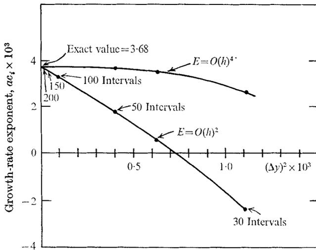
FIGURE 3. The effect of channel resolution on the accuracy of linear solutions ( $\alpha = 1$ ,  $R = 10000$ ).
