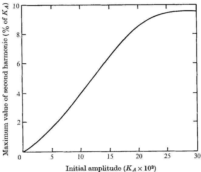
FIGURE 8. The effect of initial amplitude on the maximum magnitude of the second harmonic.
