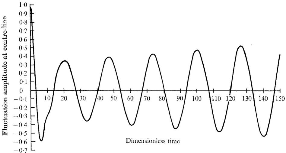
FIGURE 2. Computed linear oscillation ( $\alpha = 1, R = 10\,000$ ).  $A(0, t) = \exp(c_i t) \cos(c_r t)$  with  $c_i = 0.003758, c_r = 0.2374$ .
